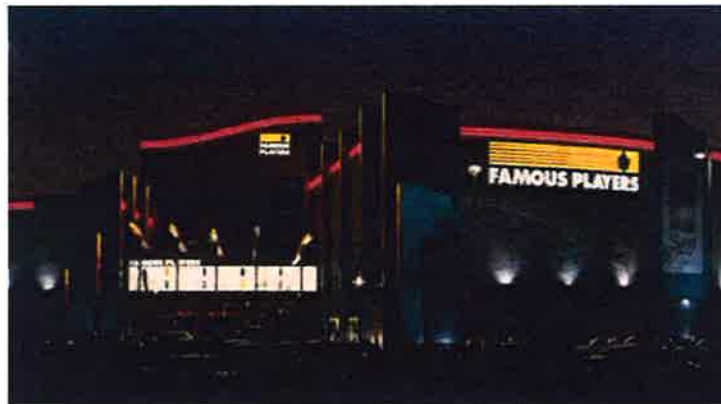
Internally illuminated pan channel fascia letters
