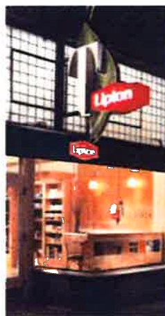
Internally illuminated three-dimensional letters
