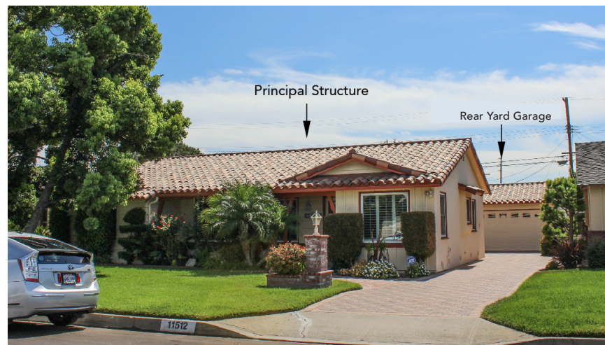
FIGURE 27: This rear yard garage does not exceed the height of the principal structure and is subordinate in massing and placement.
