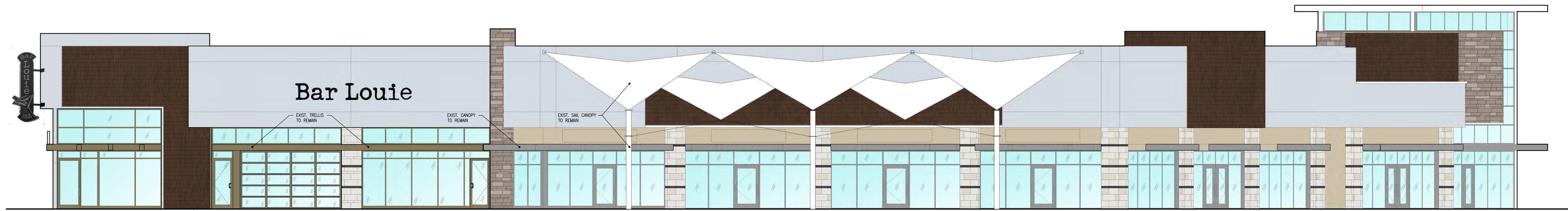
⊕ A1.402 EXISTING EXTERIOR ELEVATION - EAST SCALE: 1/8"=1'-0"
