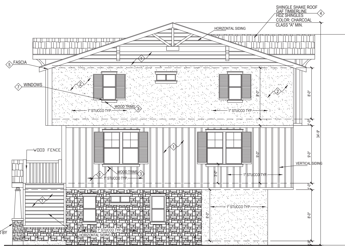
SOUTH ELEVATION (BUILDING 1) UNIT 1 & 2 SCALE 1/4"=1'-0"
