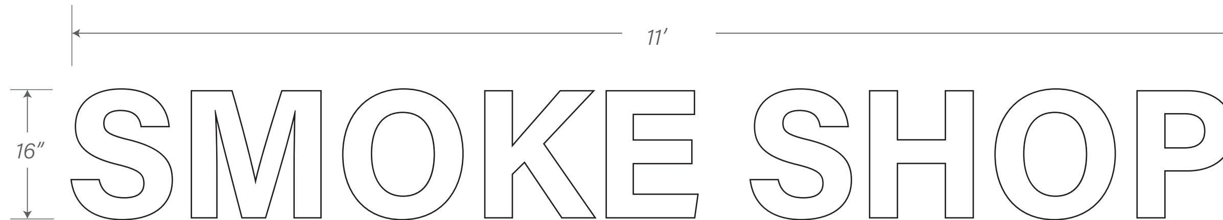
PRIMARY SIGN TYPE - INTERNALLY ILLUMINATED CHANNEL LETTERS
