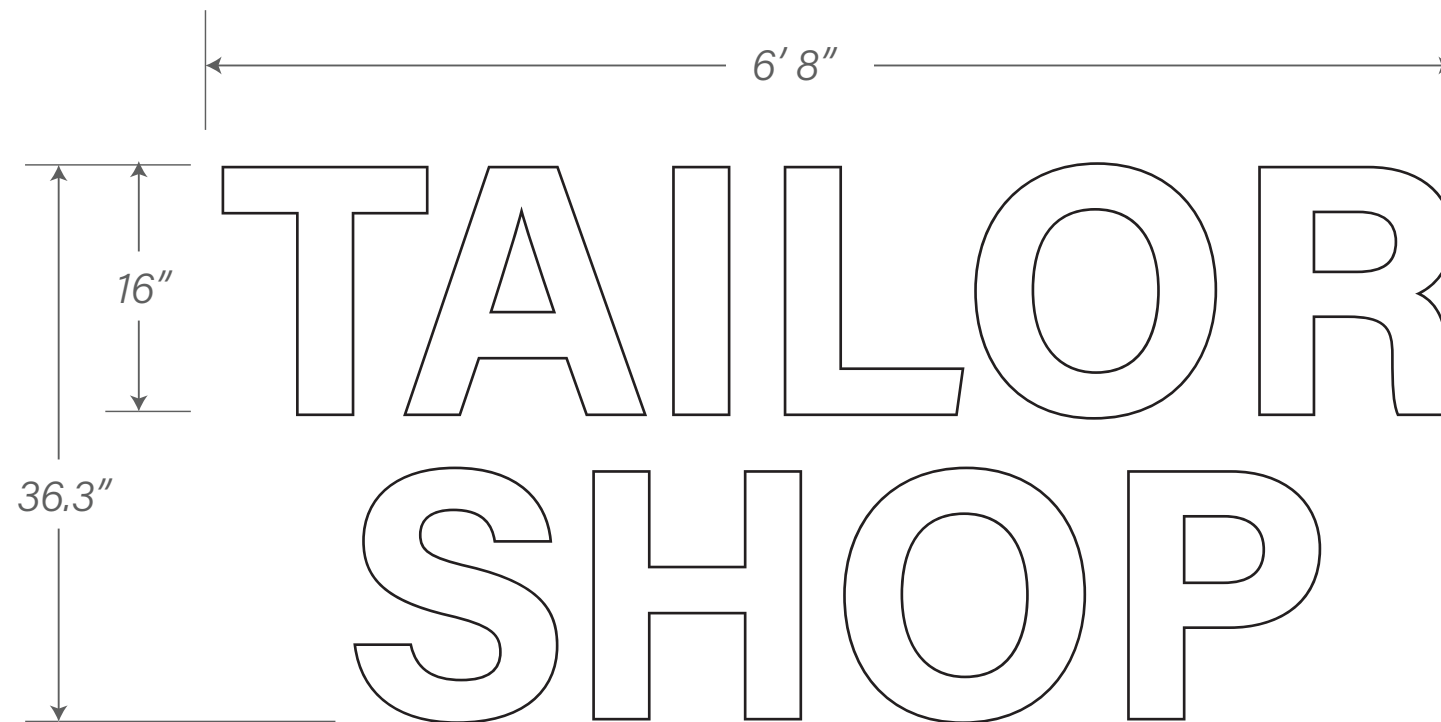
PRIMARY SIGN TYPE - INTERNALLY ILLUMINATED CHANNEL LETTERS
