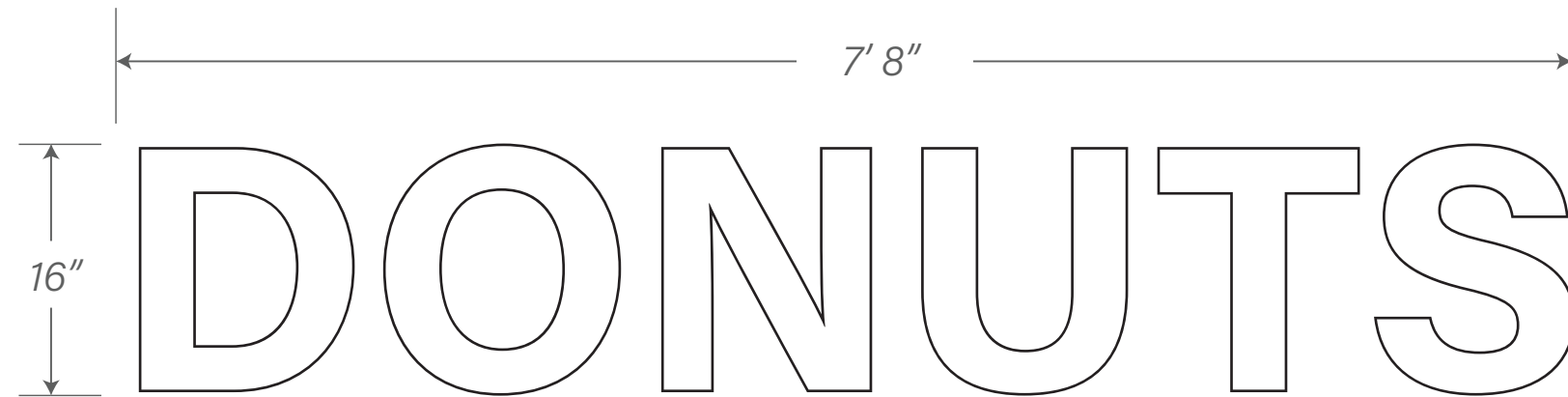
PRIMARY SIGN TYPE - INTERNALLY ILLUMINATED CHANNEL LETTERS
