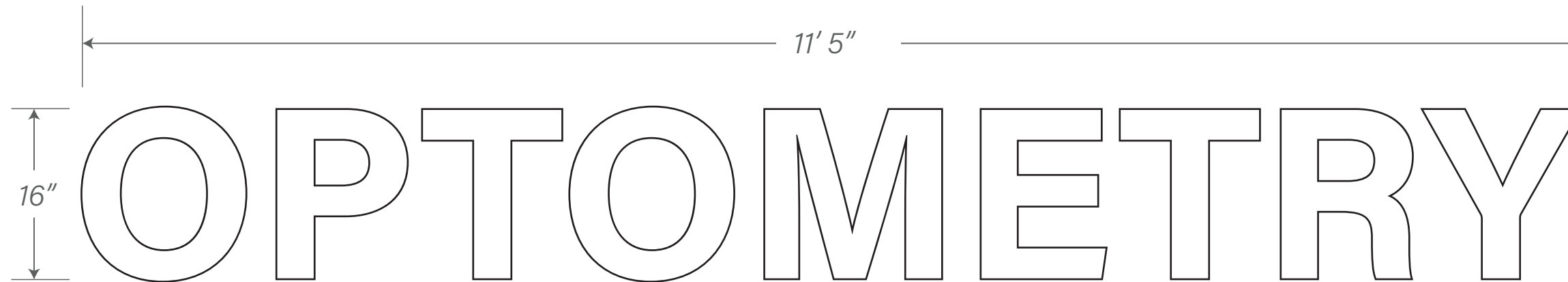
PRIMARY SIGN TYPE - INTERNALLY ILLUMINATED CHANNEL LETTERS
