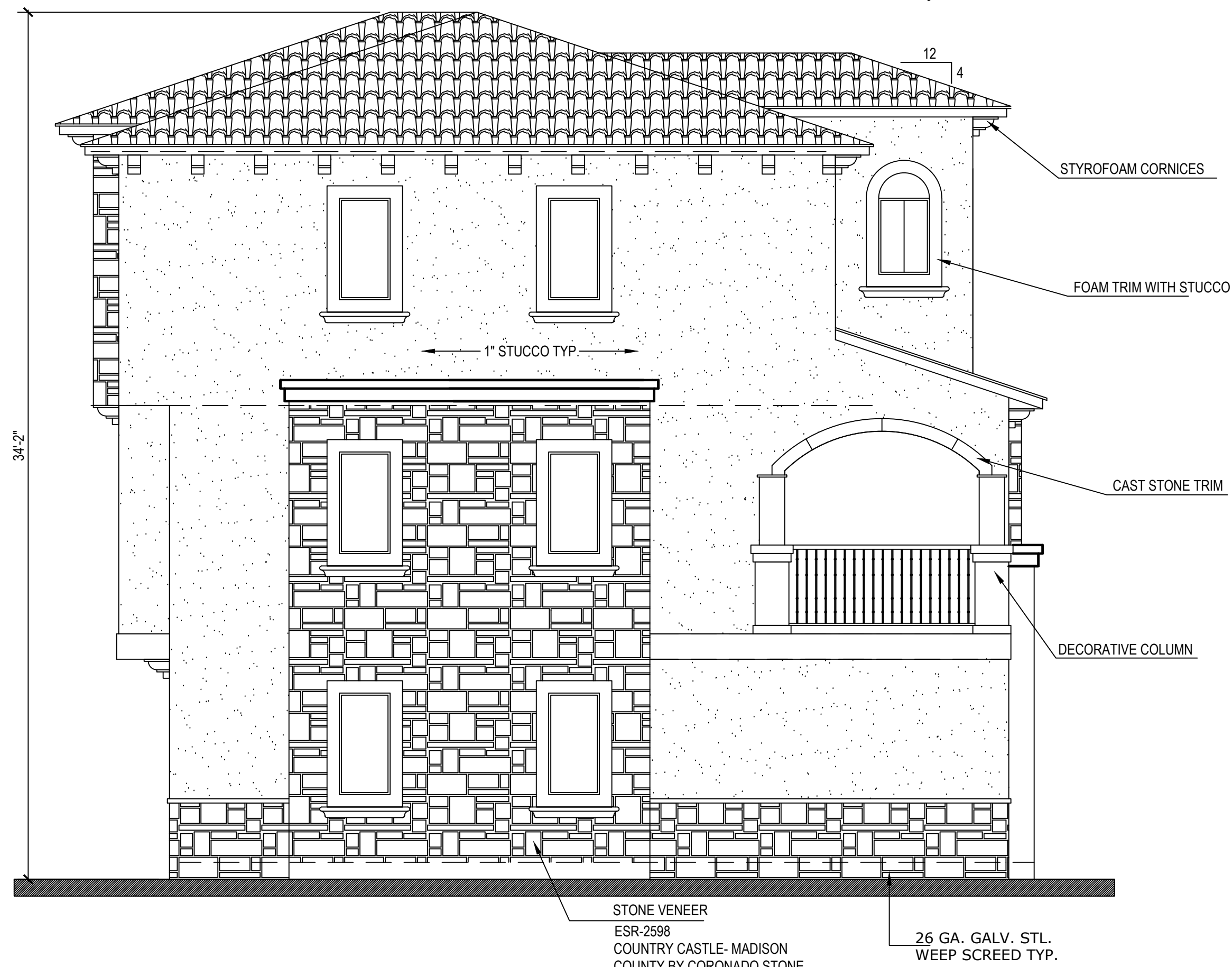
NORTH ELEVATION (BUILDING 1) UNIT 1 & 2 SCALE 1/4"=1'-0"
