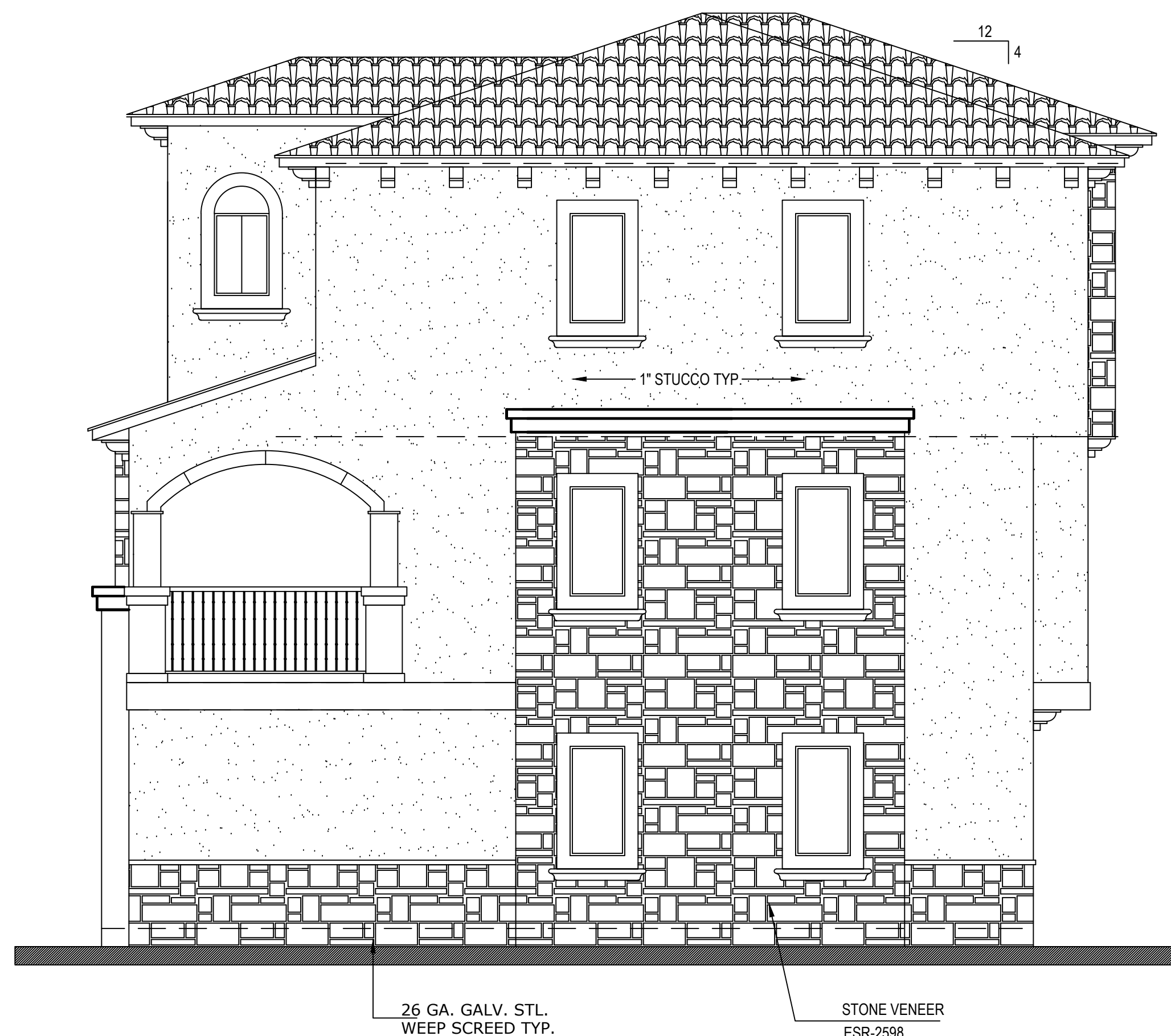
SOUTH ELEVATION (BUILDING 1) UNIT 1 & 2 SCALE 1/4"=1'-0"
