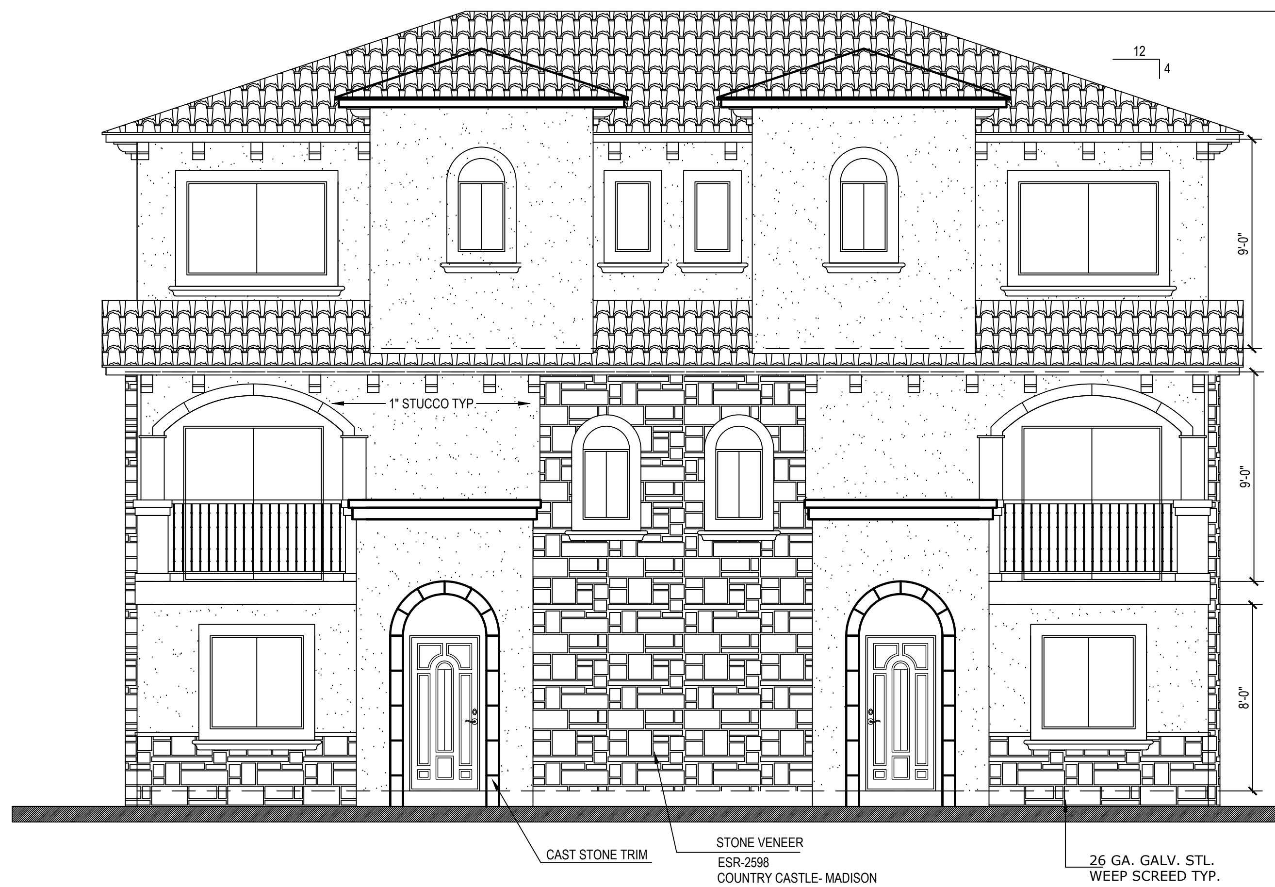
WEST ELEVATION (BUILDING 1) UNIT 1 & 2 SCALE 1/4"=1'-0"
